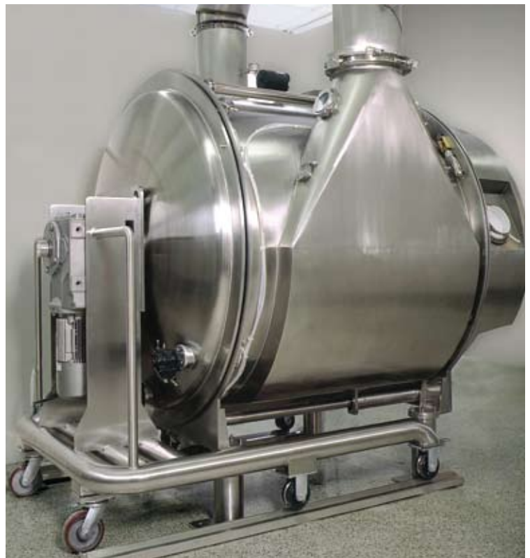
Farr containment dust collectors pull dust off of tablet coaters like this Spectrum Coater from Thomas Engineering
